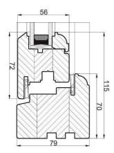
The INLINE CASEMENT is specifically designed to replicate a period window whilst incorporating the latest modern operation and security features. Often referred to as a conservation window, the design is characterised by a sash that sits within the frame to create a flush finish externally, the perfect choice for listed properties.
