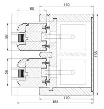
The **SLIDING SASH CORDS & WEIGHTS** window utilises pulleys and weights as the lift system. Primarily used when build circumstances dictate or when conservation requirements are a consideration. Ensuring the character and charm of the building is maintained whilst incorporating modern technologies, security and performance.
